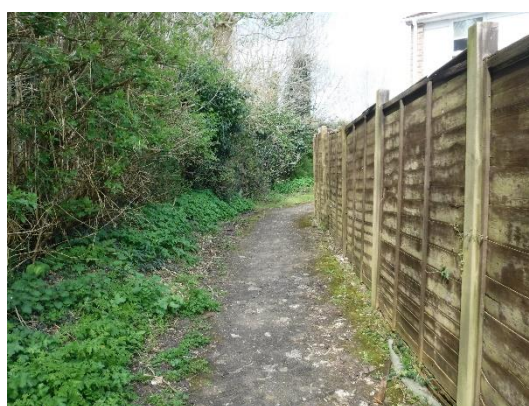
Figure 5.2 Urban pedestrian footpaths need to be sealed-surfaced, with good forward sight lines and lighting to feel safe at night. Where they connect cul-de-sacs or otherwise improve permeability, they should be constructed to shared path dimensions (not less than 3.0m) or segregated if the path has a higher volume of pedestrians.
