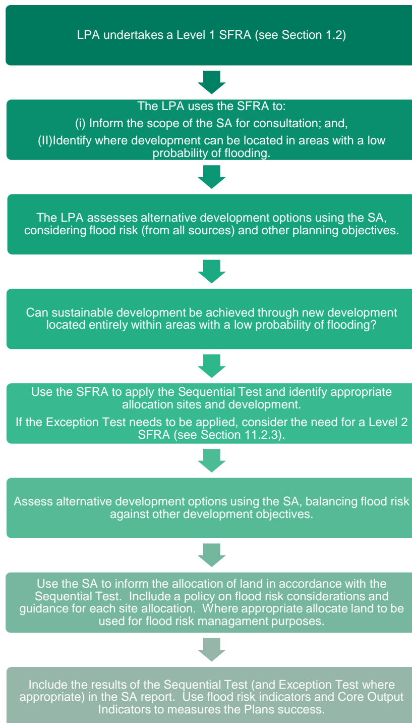
Figure 1-1 Taking flood risk into account in the preparation of a Local Plan (Planning Practice Guidance for Flood Risk and Coastal Change)
