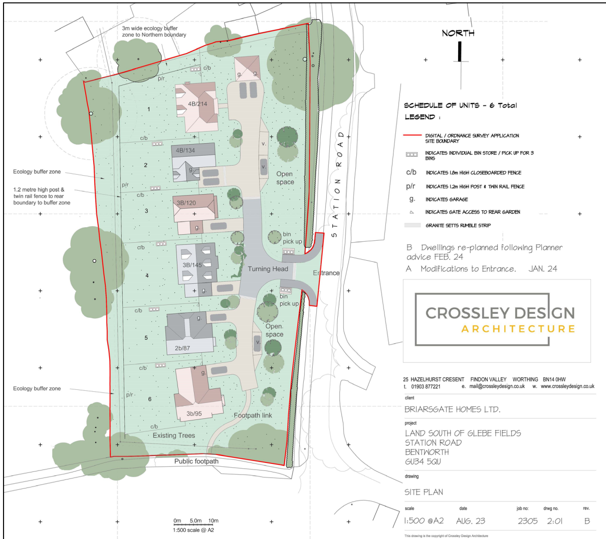
Fig. 2 Site Plan for Planning Application Ref. 60094 to Develop Allocation BWH1 with 6 Dwellings
